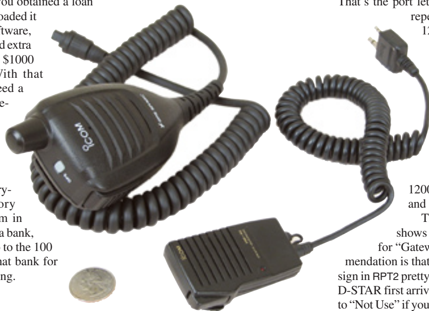
Figure 5 — The HM-175GPS speaker/mic includes a GPS receiver, making a self-contained package. It's big, as shown here with a more conventional speaker/mic.
