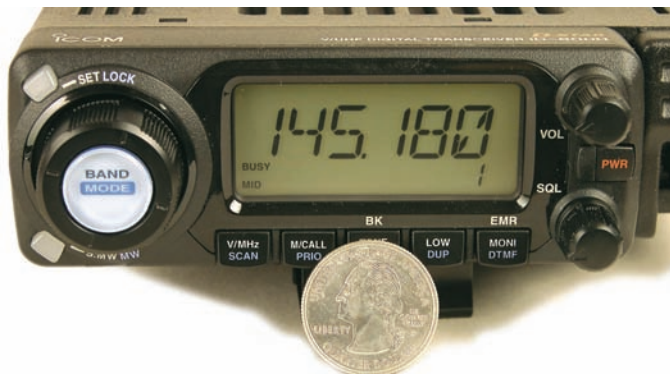
Figure 3—The ID-800H control head packs a lot of features into a small space. Dual-purpose push buttons control most of the commonly used functions, while many others are selected via the set menu.
